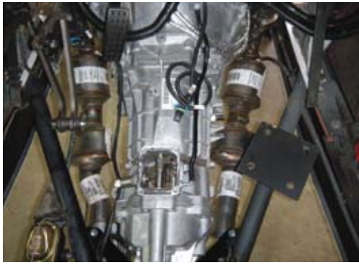
GM catalytic converters were installed in the SO-CAL Speed Shop '32 Ford roadster. Shown is the clearance for the clutch and brake pedal assembly.
