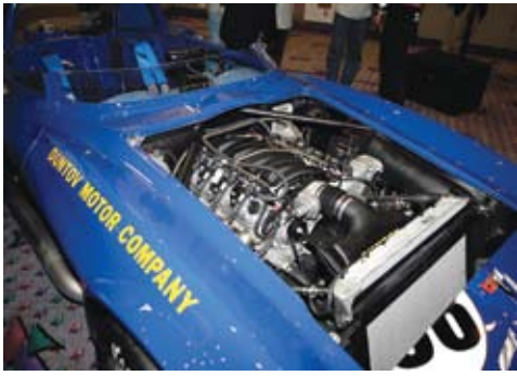
A GM E-ROD LS engine installed in a replica Chevrolet Corvette Grand Sport from Duntov Motor Co.
