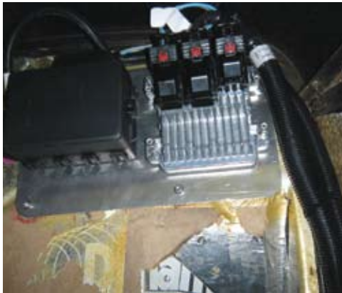
The GM ECM included in the E-ROD package installed in the SO-CAL '32 Ford roadster.
