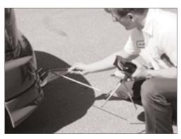
SEMA-model legislation provides for the testing of exhaust noise through a standard (J1169) adopted by the Society of Automotive Engineers. To be certified under the SEMA model, vehicles may not exceed 95 decibels.
